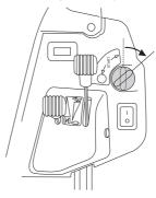
6 When the engine starts release the ignition key immediately back to neutral position.
